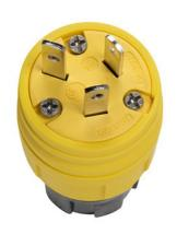
Rated watertight for 1,500 psi high-pressure hosedown, Pass and Seymour plugs and connectors feature multiple seals to ensure protection against the environment. Constructed of a sturdy rubber body, which makes them impact- and chemical-resistant, they have nickel-plated blades and contacts for superior corrosion resistance.
