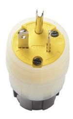
Rated watertight for 1,500 psi high-pressure hosedown, Pass and Seymour watertight plugs and connectors feature multiple seals to ensure protection against the environment. Thermoplastic elastomer (TPV) construction stands up to impacts, oils, chemicals, heat and weather.
