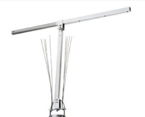
Drop Ceiling Support with single #10 support for 24-36\\ spans, 38\\ drop.
