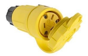
Rated watertight for 1,500 psi high-pressure hosedown, Pass and Seymour plugs and connectors feature multiple seals to ensure protection against the environment. Constructed of a sturdy rubber body, which makes them impact- and chemical-resistant, they have nickel-plated blades and contacts for superior corrosion resistance.
