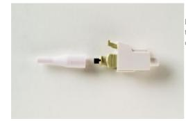
Legrand quick-cure, anaerobic epoxy field-installable connectors speed installation time. Strip the fiber, inject the adhesive into the connector, insert and scribe the fiber, then polish the connector end face to perfection for a high performance termination.
