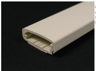
Wiremold 2300 Series Raceway is a low-profile, two-piece raceway with durable, textured PVC white finish. Available in 5' (1.52m) lengths. Packed 50' (1.5sm) per carton. Supplied with wide adhesive tape along its entire length.
