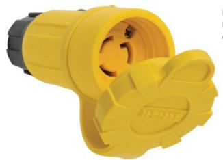
Locking Watertight Connector, 15amp 125volt, NEMA Configuration L5-15, multipoint sealing system provides environmental protection of NEMA 4, 4X, 6, 6P, and IP67 rated.
