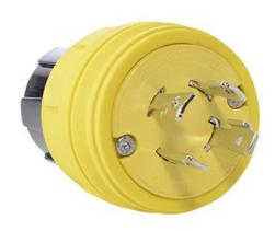
Locking Watertight Plug, 30amp 3 480 volt, NEMA Configuration L16-30, multipoint sealing system provides environmental protection of: NEMA 4, 4X, 6, 6P and IP67 rated.
