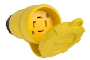
Locking Watertight Connector, 30amp 3 250volt, NEMA Configuration L15-30, multipoint sealing system provides environmental protection of NEMA 4, 4X, 6, 6P, and IP67 rated.
