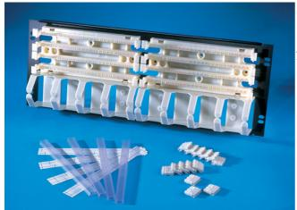
Legrand® 110 Block Panels provide two 100-pair block kits and two jumper troughs (without legs) on a 19"W panel that is mountable to the Mighty Mo® rack system or to other EIA racks.
