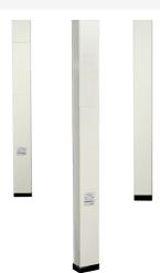
Single-compartment pole. Nominal material thickness .040" [1.0mm]. Furnished unwired without outlets. Mounting hardware, entrance end fitting and ceiling trim plates furnished. Length: 12'5" [3.8m].
