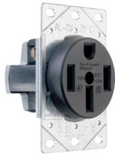
A durable solution that provides 50A 125/250V NEMA 14-50R power access for ranges, dryers and electric vehicle (EV) chargers. A single, flush-mount, straight-blade receptacle. 3-Pole, 4-Wire.
