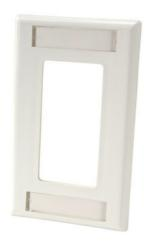
Series II Single Gang Faceplate accepts a wide variety of Series II modules. Plate provides three units of module space and is .75" deep, cloud white. Legrand® offers single and double gang Series II® plastic faceplates with a variety of module capacities to match your workstation applications. Series II plates offer recessed label fields, slotted screw holes to adjust alignment and are ruggedly constructed from high impact thermo-plastic 94V-0 rated to ensure long life.
