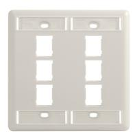
HDJ faceplates are available in 1, 2, 3, 4 & 6 port in a single gang and 6 & 12 port in a double gang. HDJ faceplates support rear load installation of HDJ copper series jacks and HDFM fiber modules. All faceplates include label fields.
