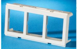
This plate accepts three TracJack modules or blanks. Use with 40700071, 40700072, or 40700073 bezels, to snap mount into 2.70" x 1.375" TIA referenced furniture openings for Steelcase, Haworth, Knoll and others
