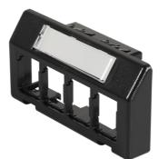
This plate has 4 rear-load jack openings for 4 high density jack (HDJ) modules or blanks. For 2.70" x 1.375" furniture openings. HDJ Furniture plates and bezels accept HDJ series jacks or modules to enable mounting in Raceways, Floor Boxes, furniture and more.
