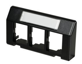
This plate has 3 Front-load jack openings for Tracjack (TJ) modules or blanks, snap mounts into  $2.70" \times 1.375"$  TIA referenced furniture openings for Steelcase, Haworth, Knoll and others.
