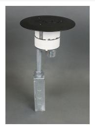
Complete with one-piece finish flange and conduit assembly. Conduit assembly consists of one 3/4" trade size conduit and one 1 1/2" trade size conduit. Finish cover flange provided with one 3/4" and one 1 1/2" trade size screw plug opening.
