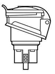
Double-Pole, 3-Wire, Pin and Sleeve International Splash-Proof Receptacle, 16A, 220/240V
