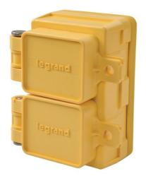
Straight Blade Watertight Duplex Receptacle, 15amp 250volt, NEMA Configuration 6-15, Impact resistant Valox lid, cover plate, and receptacle body withstand impacts, chemical, and corrosion.
