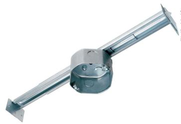
Slide fan support - same heavy-duty slide as 55501, but with 2.0-inch deep box, to accommodate up to 1-inch firewall or soundproofived ceilings, with rotating dual support for 16-24-inch spans, bulk packed. 25-Pack.
