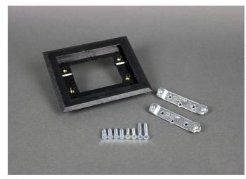
One gang black nonmetallic carpet flange, for OmniBox® and Modulink<sup>™</sup> Series floor boxes. Accepts a 6A communication adapter (CM-MAB), and Ortronics MAB3S2 and MAB6TJ adapters. NOTE: Brass covers and flanges are not interchangeable with aluminum or nonmetallic covers and flanges. Nonmetallic covers are interchangeable with aluminum flanges.
