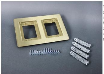
Two gang brass combination carpet and tile flange, for OmniBox® and Modulink™ Series floor boxes. Flange is 6.080 inch x 9.185 inch (154.4mm x 233.3mm). Accepts Ortronics MAB6TJ TracJack and MAB3S2 Series II, and Wiremold CM Series Open System adapters, sold separately. NOTE: Brass cover plates can only be used with brass flanges. Brushed aluminum flanges come with beveled edges.
