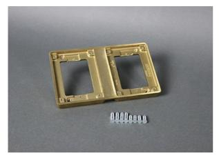
Two-gang brass tile flange, 4.524" x 7.624" (107.0mm x 193.7mm). For use on 880S2, 880M2, 880CS2-1, and 880CM2-1 Floor Boxes. NOTE: Brass covers and flanges are not interchangeable with aluminum or nonmetallic covers and flanges. Nonmetallic covers are interchangeable with aluminum flanges.
