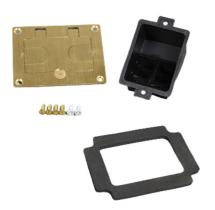
Brass communication cover plate. Allows for up to four communication devices to be mounted in a recessed position within the 880S and 880CS Floor Boxes. Has removable slides for cable egress. NOTE: Not for use with 817C, 827C, and 837C Flanges.
