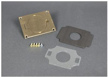
Brass single locking receptacle cover plate. Single flip lid cover for 20A or 30A single locking receptacles. Device opening is 2 5/8" (67mm). For use with maximum female locking device of 1.58" diameter, and maximum male plug face of 2.25" diameter. NOTE: Brass covers and flanges are not interchangeable with aluminum or nonmetallic covers and flanges. Nonmetallic covers are interchangeable with aluminum flanges.
