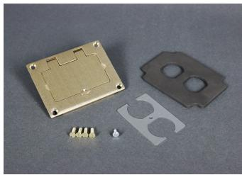
Brass rectangular cover plate, 3.156" x 4.182" (80.2mm x 106.2mm). Allows for mounting of a duplex style receptacle with a rectangular style flip lid cover.
