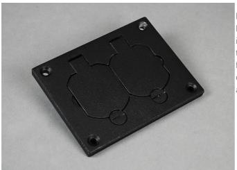
Black powdercoat duplex cover plate, for OmniBox® and Modulink™ Series floor boxes. Cover plate is 3.290 inch x 4.310 inch (83.6mm x 109.5mm). Flip lids can also be used with 106 type frames for communications. NOTE: Brass covers and flanges are not interchangeable with aluminum or nonmetallic covers and flanges. Nonmetallic covers are interchangeable with aluminum flanges.
