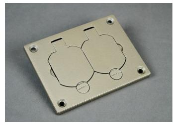
Nickel powdercoat duplex cover plate, for OmniBox® and Modulink<sup>™</sup> Series floor boxes. Cover plate is 3.290 inch x 4.310 inch (83.6mm x 109.5mm). Flip lids can also be used with 106 type frames for communications. NOTE: Brass covers and flanges are not interchangeable with aluminum or nonmetallic covers and flanges. Nonmetallic covers are interchangeable with aluminum flanges. Made in USA.
