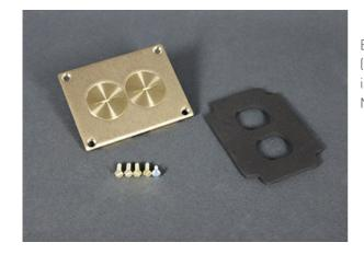
Brass duplex cover plate, screw plugs. Screw plugs are 1 1/2" (38mm) in diameter. NOTE: Brass covers and flanges are not interchangeable with aluminum or nonmetallic covers and flanges. Nonmetallic covers are interchangeable with aluminum flanges.
