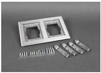
Two gang brushed aluminum combination carpet and tile flange, for OmniBox® and Modulink™ Series floor boxes. Flange is 5.940 inch x 9.045 inch (150.9mm x 229.7mm). Accepts Ortronics MAB6TJ TracJack and MAB3S2 Series II, and Wiremold CM Series Open System adapters, sold separately. NOTE: Brushed aluminum flanges come with beveled edges. Brass cover plates can only be used with brass flanges. Brushed aluminum flanges come with beveled edges.
