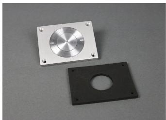
Brushed aluminum power or communications cover plate with 2" and 1"trade size plugs. Acceptable for use with threaded conduit when passing through power cables. NOTE: Brass covers and flanges are not interchangeable with aluminum or nonmetallic covers and flanges. Nonmetallic covers are interchangeable with aluminum flanges.
