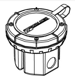
Die-cast aluminum construction with three 1/2"" (12.7mm) knockouts, two on the sides and one on the bottom. 18 cu. in. (295ml3) of capacity. Requires a 4"" (102mm) diameter hole. Comes complete with a disposable cover, receptacle and cover sold separately.
