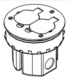
Complete with 20A duplex receptacle and brass cover plate. Die-cast aluminum construction with three 1/2'' (12.7mm) knockouts. Two on the sides and one on the bottom. 18 cu. in. (295ml3) of capacity. Requires a 4'' (102mm) diameter hole.
