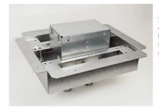
2-Gang Fire Classified Steel Floor Box. Adjustment range over deck of 2" (51mm) minimum to 6-1/2" (165mm) maximum. One 1 1/4" (32mm)and One 2" (51mm) conduit feed openings. Box Capacity -58.5 cubic inches each gang. This floor box preserves up to a 3-hour fire rating of floors in which it has been installed.
