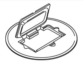
The Wiremold Ratchet-Pro™ brass GFI cover plate with decora flip lid, 5 1/2 inch (140mm) for carpet or tile installations. Cover also works with 880 Series™ boxes. NOTE: All cover plates are furnished with gasket and three screws.
