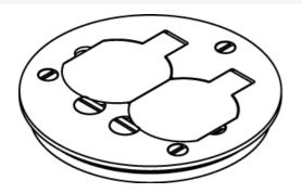
Brushed aluminum duplex cover plate with flip lids, 4 1/4" (108mm) for tile. NOTE: For carpet or tile installations. All cover plates are furnished with gasket and three screws. The 895P Polycarbonate Series Cover Plates must be field modified for dual service.
