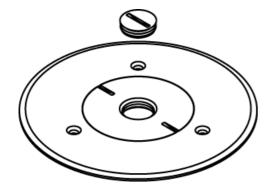
Brass cover plate with 1/2" (12.7mm) threaded opening 5 1/2" (140mm) for carpet. NOTE: For carpet or tile installations. All cover plates are furnished with gasket and three screws. The 895P Polycarbonate Series Cover Plates must be field modified for dual service.
