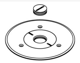
Brass cover plate with 3/4" (19.1mm) threaded opening for carpet. NOTE: For carpet or tile installations. All cover plates are furnished with gasket and three screws. The 895P Polycarbonate Series Cover Plates must be field modified for dual service.
