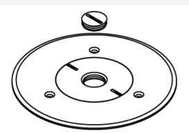
Brushed aluminum (896CKAL-1/2) cover plate with 1/2" (12.7mm) threaded opening 5 1/2" (140mm) for carpet. NOTE: For carpet or tile installations. All cover plates are furnished with gasket and three screws. The 895P Polycarbonate Series Cover Plates must be field modified for dual service.
