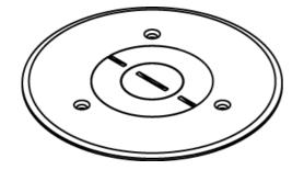
Polycarbonate communications or power cover plate. Includes one plug with 3/4'' (19mm) opening, one plug with 1'' (25mm) opening, and one plug with 2 5/8'' (67mm) opening. For pass-through only. NOTE: For carpet or tile installations. All cover plates are furnished with gasket and three screws. The 895P Polycarbonate Series Cover Plates must be field modified for dual service.
