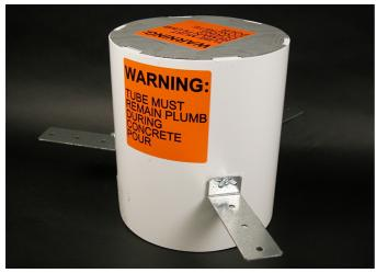
Nonmetallic sleeve attaches to structural decking and maintains 8'' - 8 1/8'' diameter cast in hole. Unit includes three (3) attachment legs, two (2) end caps and three (3) thumb screws.
