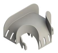
Use Over-the-Top Waterfall for cables that exit or enter the side of the tray. It eliminates the need to cut any side wires that reduce tray integrity. Over-the-Top Waterfall features steel, powder coated construction and hold-down slots to zip tie cables in place.
