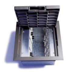
With a 5 inch (127mm) depth, the AC Series™ AC10105 Raised Floor Box provides eight gangs of power and/or communication device capacity. Power plate with duplex knockouts included with box. It also provides increased plug-in volume which is ideal for the additional space needed when plugging in transformer type plugs. Lids can be rotated 180° for easy orientation. Gray lids are die-cast zinc construction, and allow for a carptet or tile insert.
