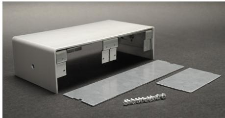
Aluminum housing and base 9 1/4" x 4 1/2" x 2 1/2" (235mm x 114mm x 64mm) are provided with four (4) 1" trade size knockouts in base for hardwiring unit and two dividers which allow units to be divided on either the "X" or "Y" axis/plane. Accommodates a variety of power (NEMA or decorator), and supports Ortronics and Wiremold Open Systems connectivity. Portals are field configurable by ordering the corresponding faceplates.
