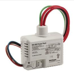
The BZ-250 power pack switches lighting or plug loads On and Off in response to low voltage control inputs, and provides up to 225mA at 24VDC to power Wattstopper occupancy sensors. It enables Manual-On sequences of operation, as well as HoldOn, Hold-Off and load shed applications when used with lighting control panels or building automation systems. This device is constructed with environmentally friendly materials and is RoHS-compliant.
