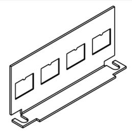
Communication bracket with four (4) RJ opening knockouts. Use as blank plate or for up to four RJ openings. Opening dimension is 9/16'' x 3/4'' (14.3mm x 19.1mm). NOTE: For use with RFB4-CI-1 only.
