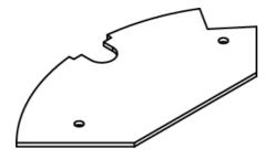
The CRFB4 has four compartments that accept different device plates. This Blank Device Plate is for Plate location 3, used to close off unused gang. NOTE: Standard size for device plates for Plate Location 3 is 5 7/32'' (132mm) x 2 3/4'' (62mm).
