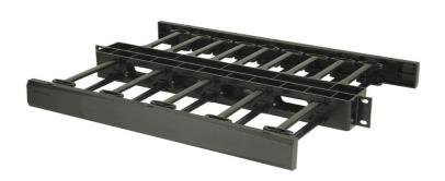
Legrand® standard horizontal cable managers are available in 1RU and 2RU sizes. Fingers begin 3/4" from the face of rack to provide bend limitation for cables, protecting cables, equipment and network performance. Included hinged cover mounts with six heavy duty clips allow them to be opened one handed without becoming "unhinged". Manufactured from UL94V-0 rated plastic.
