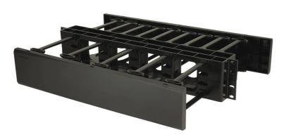
Legrand® standard horizontal cable managers are available in 1RU and 2RU sizes. Fingers begin 3/4" from the face of rack to provide bend limitation for cables, protecting cables, equipment and network performance. Included hinged cover mounts with six heavy duty clips allow them to be opened one handed without becoming "unhinged". Manufactured from UL94V-0 rated plastic.
